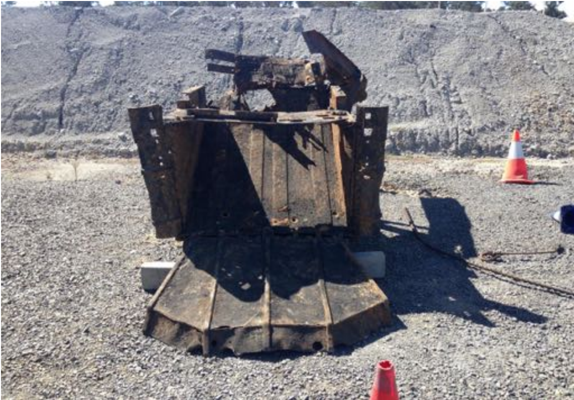
Figure 34: Scraper loader uncovered in the former Werris Creek Coal Mine in 2012. This is probably one of the scraper loaders introduced to the mine during modernisation in 1949
