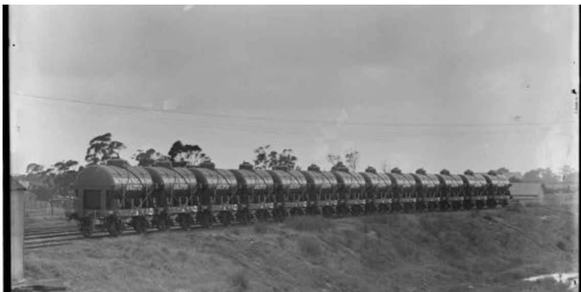
Figure 37: 13 standard gauge, 4-wheel, railway tank wagons, Nos 3 to 15, built by Clyde Engineering Pty Ltd in Granville circa 1912 for the British Australian Oil Co. Ltd. They carried Temi oil shale from Murrurundi to Hamilton near Newcastle. The tank wagons were indirectly acquired by the NSW Government Railways and numbered in the railways' L (Loco) and W (Way and Works) series and appear to have been used to carry water. Museum of Applied Arts and Sciences.
